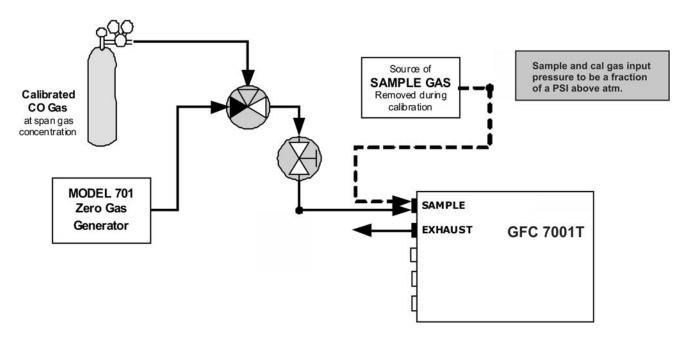
Figure 3-18: Pneumatic Connections-Basic Configuration-Using Bottled Span Gas
